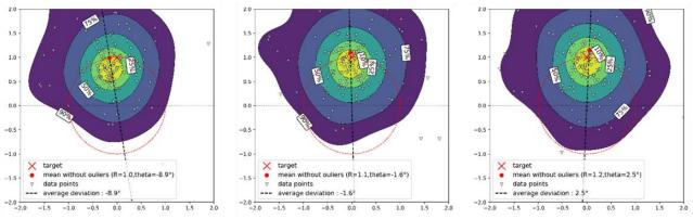
Above: One-day long simulations of 10 icebergs in the West Greenland Sea using three different inputs for ocean currents and represented in scaled polar coordinates (speed and veering angle). When icebergs are further than 20 km from the coast, the simulations are able to simulate the speed (distance from the center close to 1) and the direction of the drift (angle compared to the vertical direction).
