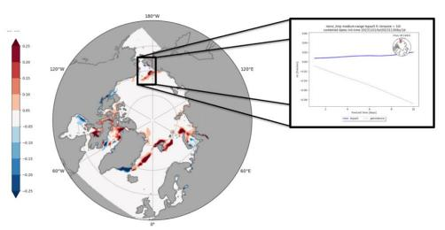
Example of plots that ICECAP can generate: sea ice concentration bias for 10-day forecasts in an ARC MFC prototype for November 2023, displayed both as a pan-Arctic map and a regional mean over the Chukchi Sea.
