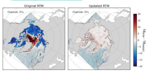
Difference between simulated and observed TB37v. TB37v is simulated with (left) the original RTM and (right) the updated RTM. AMSR2 and ERA5 data are used as input in the RTM simulation. Period of simulation is January 2024.
